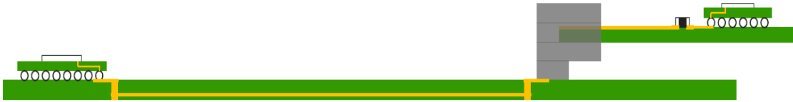
Figure 19 – Typical FC-PI-6 electrical channel construction
