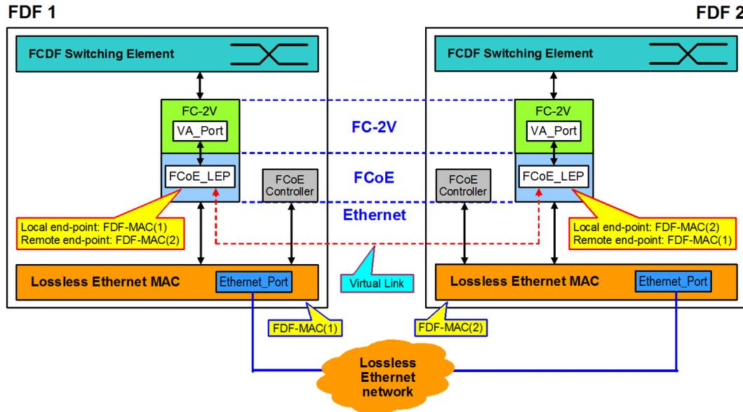
Figure 50 – VA\_Port to VA\_Port Virtual Link Example
