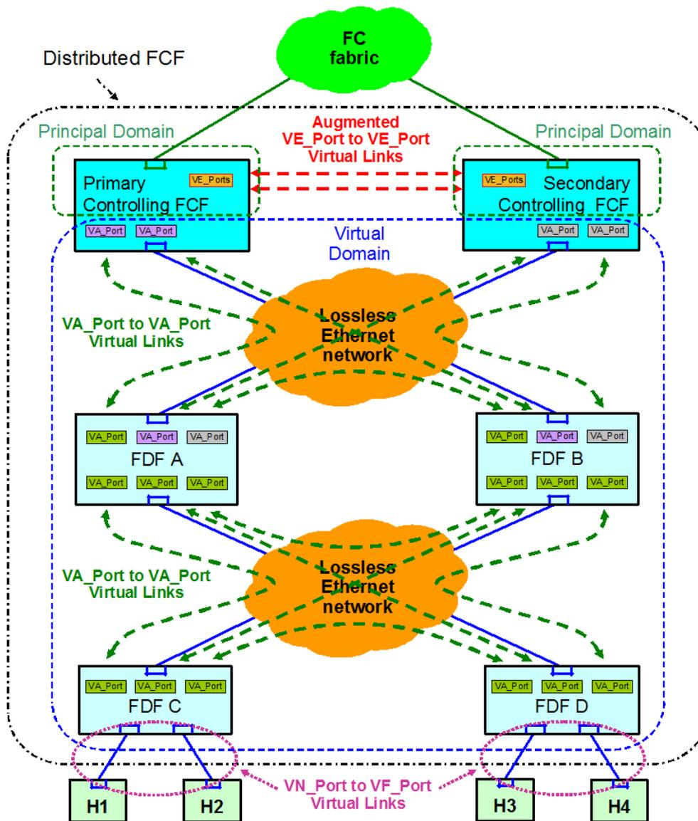
Figure 47 – Example of Distributed FCF with cascaded FDFs example
