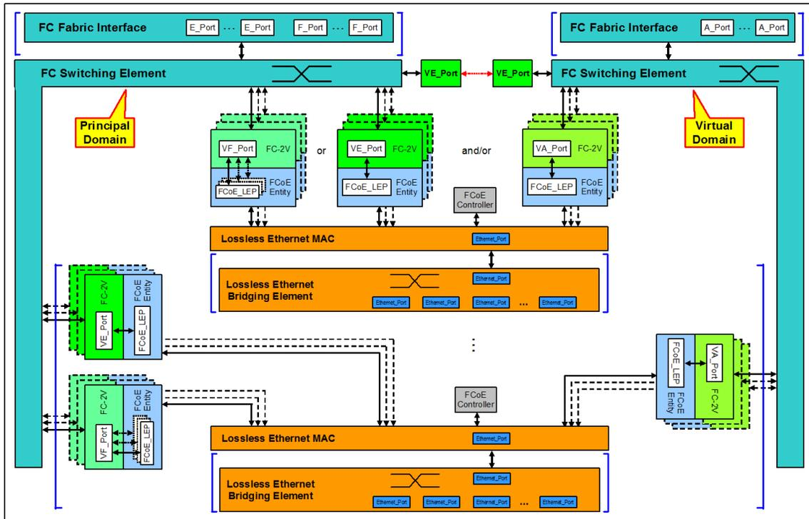
Figure 48 – Controlling FCF Functional Model
