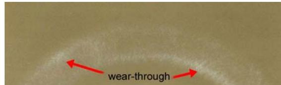
**Figure 19 - Surface wear-through**
