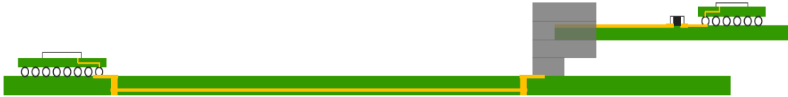
Figure C.1 – Typical FC-PI-7 electrical channel construction
